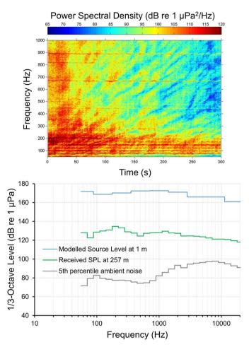
Fig. 3. Spectrogram at the closest point of approach for the Awanuia in New Zealand (top, distance = 257 m), and its corresponding 1/3-octave spectra along with the estimated source level spectra and 5th percentile ambient noise levels (bottom).
