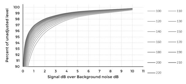
Figure 1. If background levels are just 3 dB under signal levels they contribute less than 3% to the total sound pressure level (less at higher levels). The different lines correspond to different sound pressure levels, the louder the noise, the smaller the contribution from less loud background noise.
