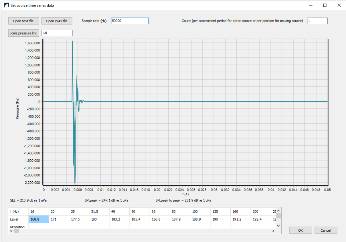
Figure 2. Example of an impulse from a 6 m diameter monopile, after import into dBSea.
