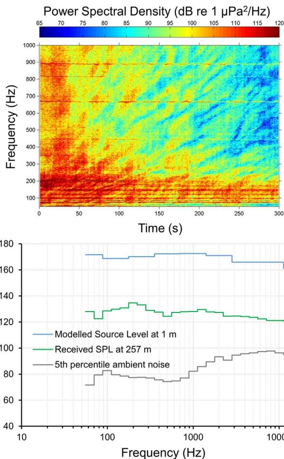
**Fig. 3.** Spectrogram at the closest point of approach for the Awanuia in New Zealand (top, distance = 257 m), and its corresponding 1/3-octave spectra along with the estimated source level spectra and 5th percentile ambient noise levels (bottom).
