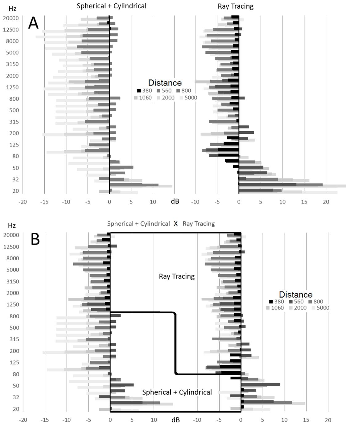
**Figure 5. Differences between measurements and model. Negative values indicate that the model predicted higher levels than were measured. A, S+CS and RT side by side for comparison, notice that S+CS gets more imprecise with increasing range, while RT is relatively inaccurate at short ranges. B, modelling employing a combination of two propagation models, crossover frequencies as marked in plot (800 Hz & 80 Hz).**
