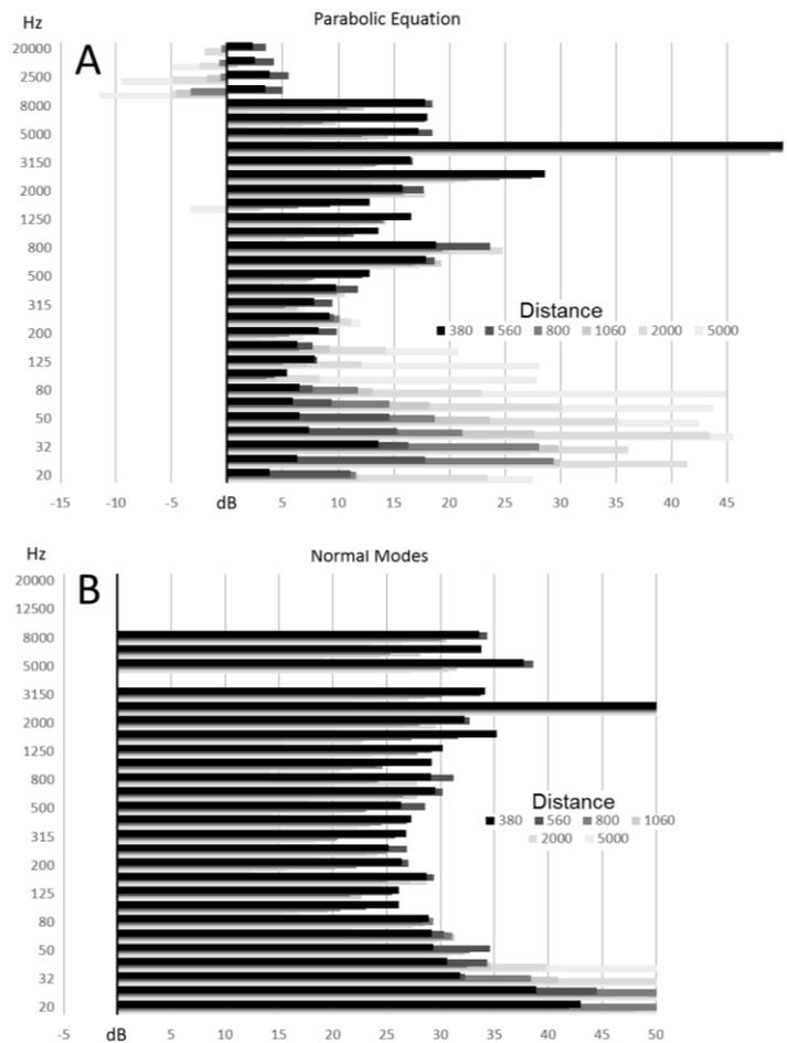
**Figure 4. Measurements minus model data in dB. Thus positive values indicate that the model predicts lower levels than the measurements. A, the PE model largely predicts levels that are lower than reality, it's especially challenged at higher frequencies. B, the NM approach appears to be unsuitable for this type of problem as model levels are very different from measured values. The lack of calculated levels at 4 kHz and above 10 kHz are due to high frequency errors.**
