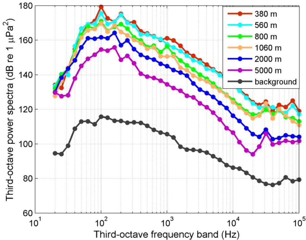
Figure 3. The third-octave band spectra for pulses at ranges from 380 m to 5 km from the driven pile. Also shown are the levels for the background noise. Reprinted with permission from [14].
