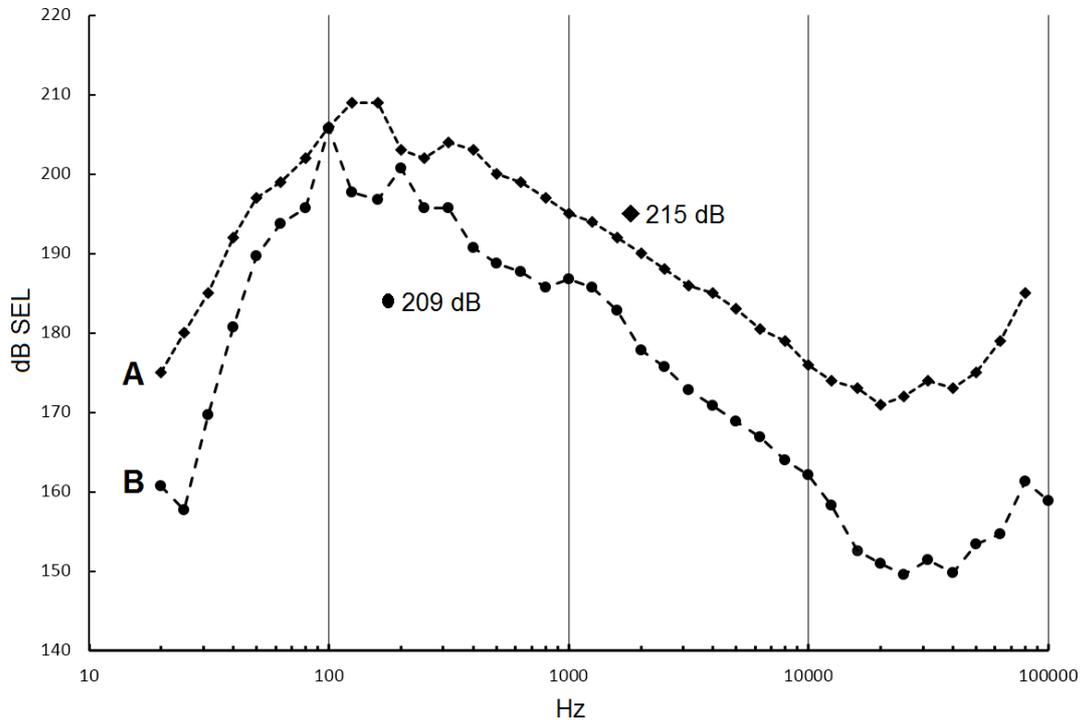
Figure 2. The two estimated source level spectrograms used for modelling noise propagation. The summated SEL value for each source is stated on graph. A, source from De Jong & Ainslie (2008). B, source from [14].
