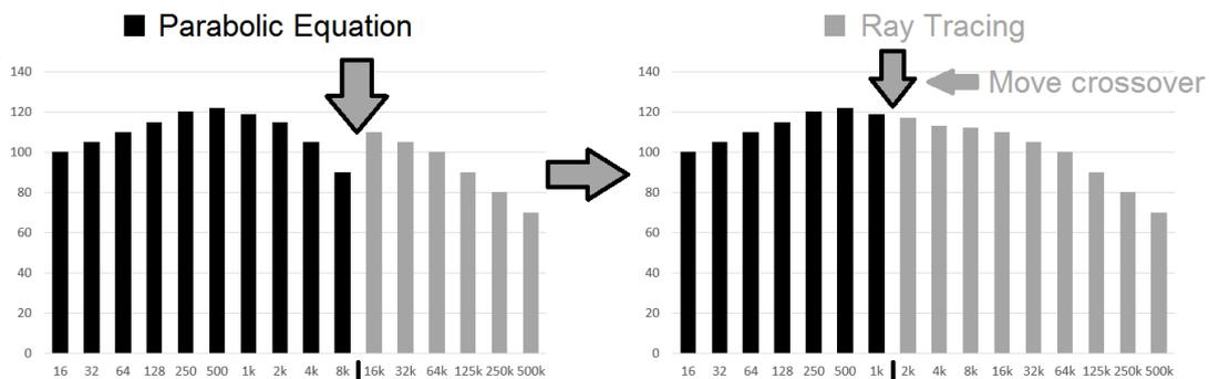
Figure 7. If received level spectrum is very different in smoothness to source spectrum, change crossover frequency.
