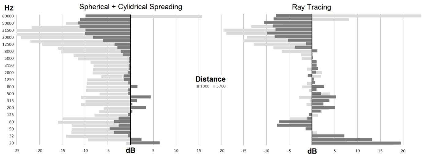
**Figure 6. S+CS and RT models difference from measurements, at two ranges. The dB values are measurement minus prediction.**
